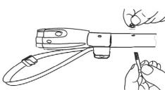
4. If you cannot use the bore as described above, then a separate hole must be drilled for mounting. For this purpose plug in the connecting piece completely until the stop (min. 40 mm deep) on the drawbar and position it in such a way that the push button is in the direction of travel to the outside (from the bike path)!
